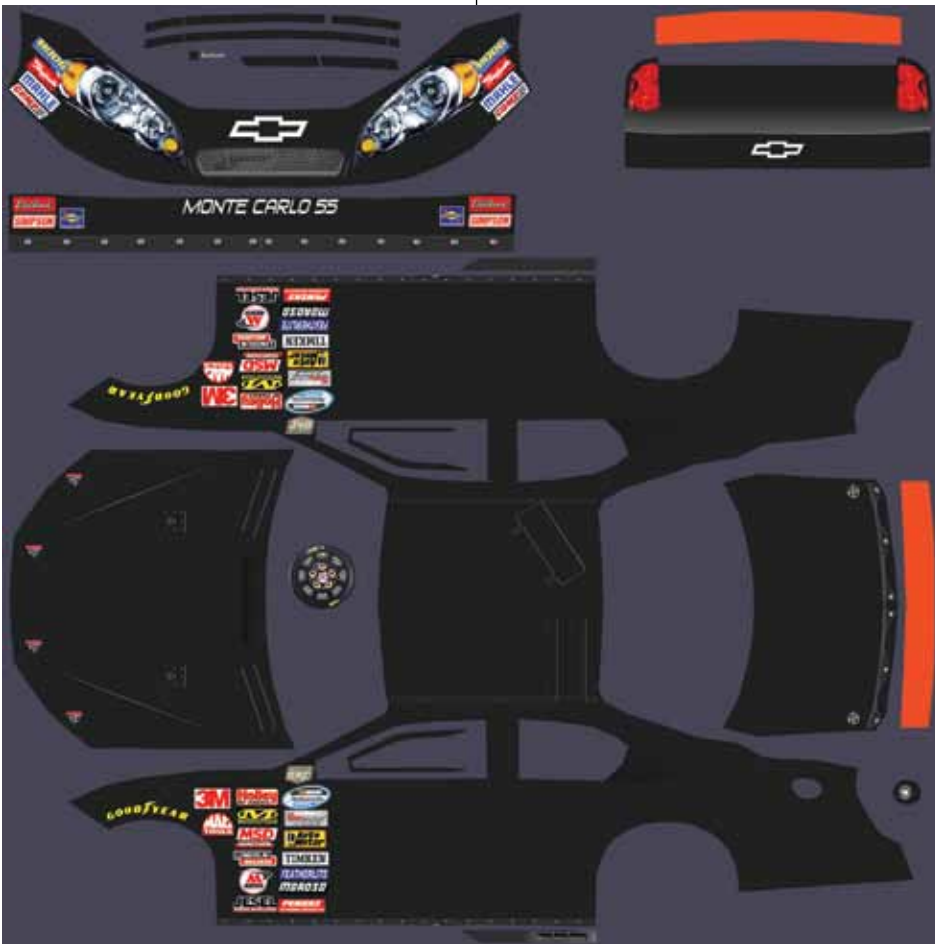
Nisbet starts his end of the design work by placing all the car's basic elements into a NASCAR-approved template, basically a race car body folded out like a broken down box.
